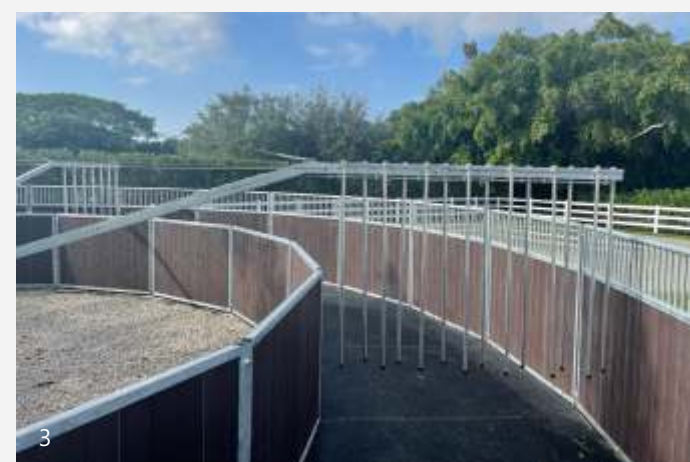
HORSE WALKER (diameter 16/4 horses) straight fence, galvanised, plastic boards
