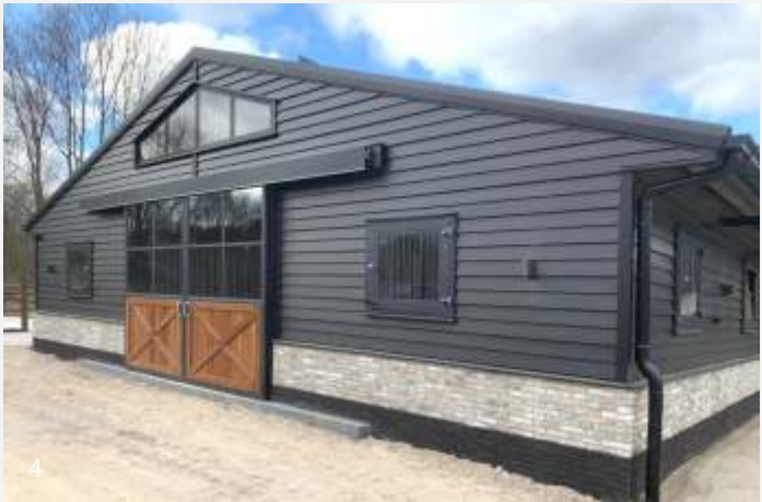
SLIDING BARN DOOR WITH SAFETY GLASS: powder coated, bamboo boards, cross in door
