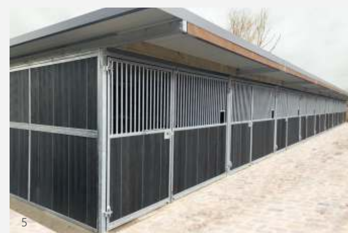
single-pitched roof, galvanised, plastic boards, hinged door, small window in door
